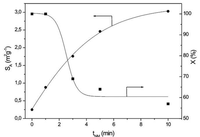
**Fig. 3.** Specific surface area  $S_A$  and content of crystalline phase X of olivine as a function of milling time  $t_{NM}$  in a nutating mill.
