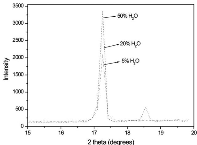
Fig. 9. XRD pattern of olivine (020) peak as a function of H<sub>2</sub>O addition by nutation milling.
