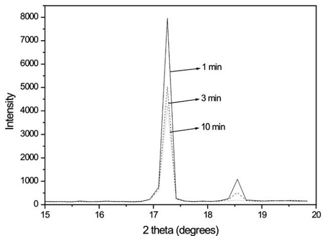
Fig. 8. XRD pattern of olivine (020) peak as a function of milling time in a nutating mill.
