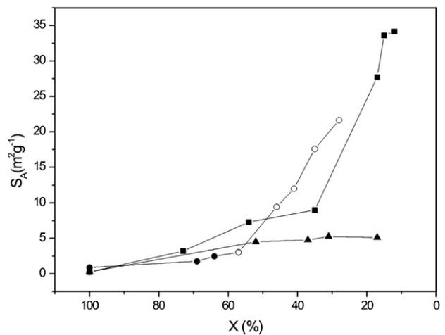
Fig. 10. Specific surface area  $S_A$  of olivine as a function of content of crystalline phase X. (■) attritor mill, (▲) planetary mill, (●) nutating mill (dry milling), (○) nutating mill (wet milling with H<sub>2</sub>O).
