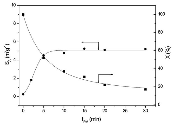
**Fig. 2.** Specific surface area  $S_A$  and content of crystalline phase X of olivine as a function of milling time  $t_{PM}$  in a planetary mill.
