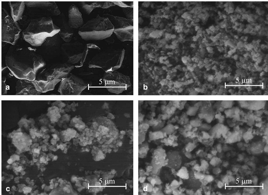
Fig. 5. SEM photographs of olivine: (a) as-received sample, (b–d) samples after milling in attritor mill, planetary mill and nutating mill, respectively.
