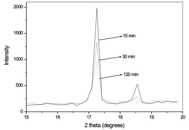
Fig. 6. XRD pattern of olivine (020) peak as a function of milling time in an attritor.
