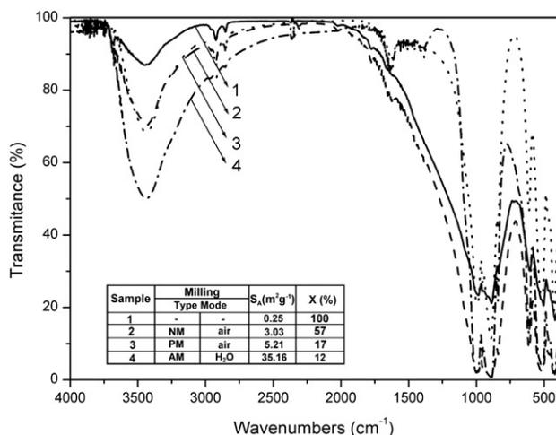
Fig. 11. FT-IR spectra of olivine: (1) initial, (2, 3, 4) after milling in planetary mill, nutating mill and attritor, respectively.
