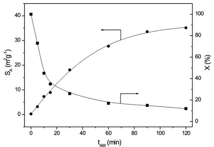
**Fig. 1.** Specific surface area  $S_A$  and content of crystalline phase X of olivine as a function of milling time  $t_{AM}$  in an attritor.
