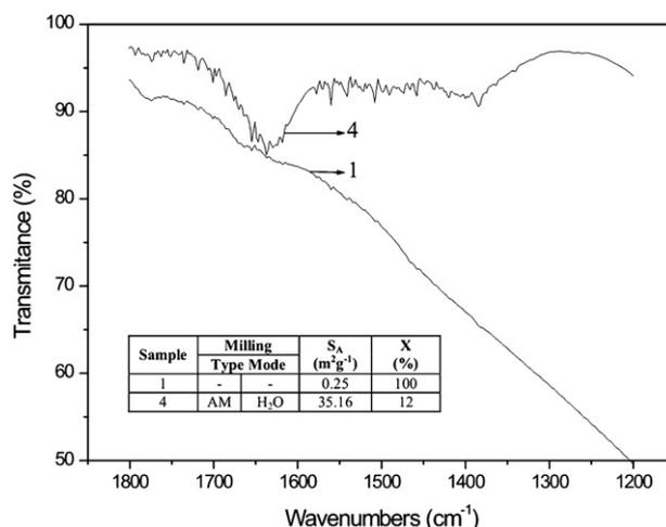
Fig. 12. FT-IR spectra of olivine: (1) initial, (4) after attritor milling. Characteristic bands for  $CO_2$  are shown.
