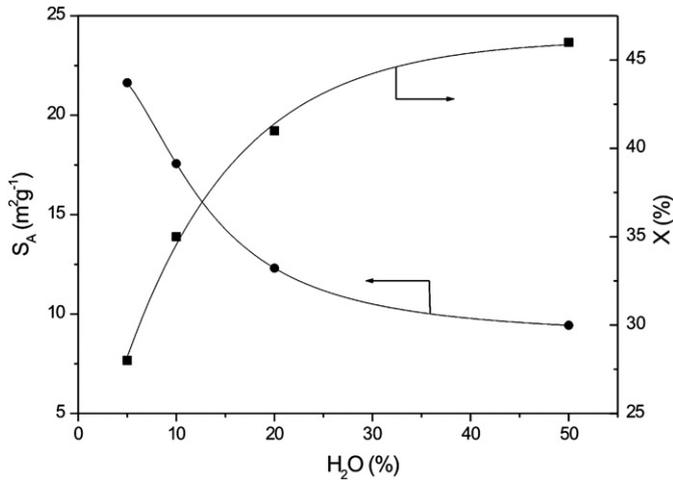
Fig. 4. Specific surface area  $S_A$  and content of crystalline phase X of olivine as a function of  $H_2O$  addition by nutating milling.
