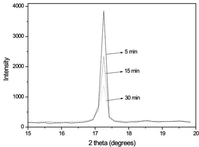
Fig. 7. XRD pattern of olivine (020) peak as a function of milling time in a planetary mill.
